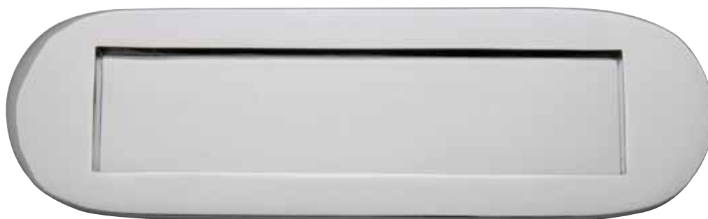
V856 Letterplate 254 x 76mm Aperture: 205 x 48mm
